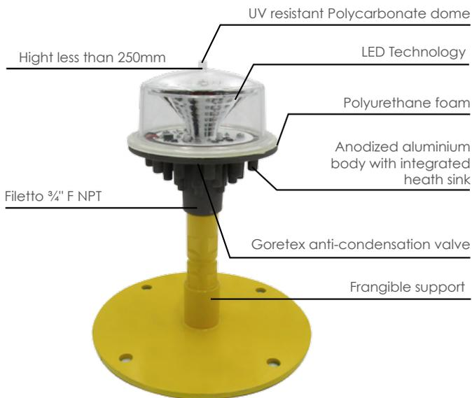
It is installed at the edges of FATO area, defining its perimeter. Alternatively, you can install the product code FATO-LXS-INSET.
